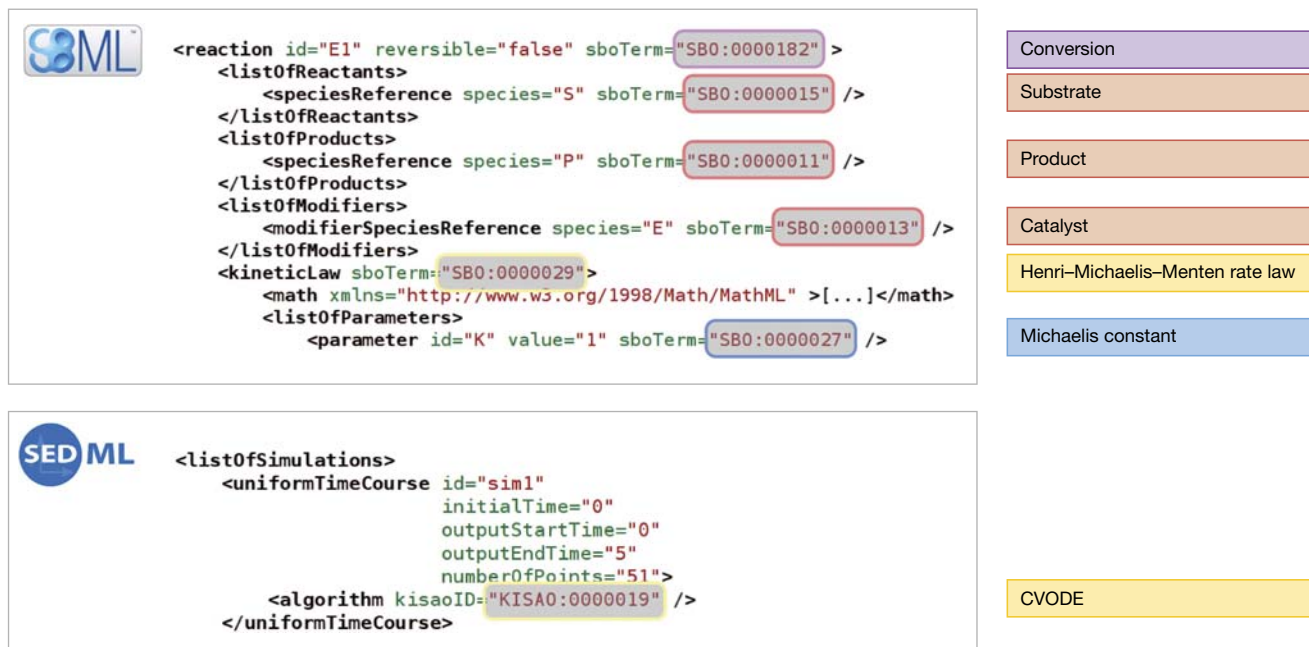
Figure 2 Use of SBO and KISAO from within SBML and SED-ML. The SBML code on the upper left makes reference to the SBO terms on the upper right. The SED-ML code on the lower left makes reference to the KISAO term on the lower right.
